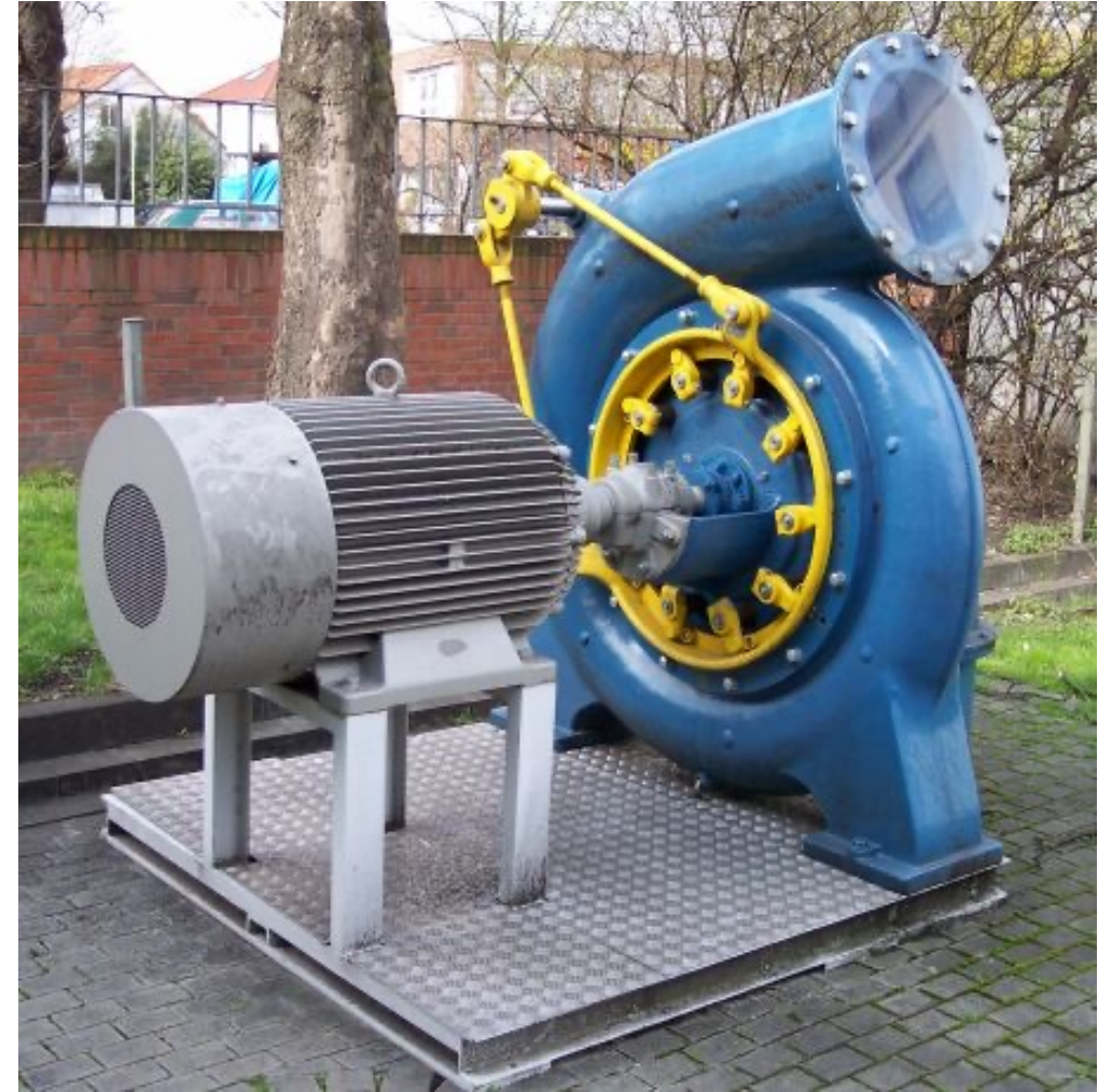
Figure 2-28: A Francis turbine connected to a generator.
